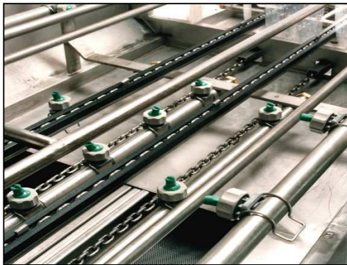
Link chains for industrial washers
