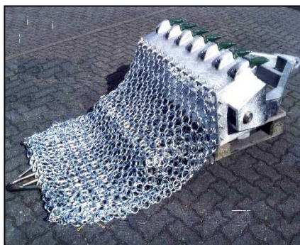
Welded chain sack (e.g. collecting purposes)
